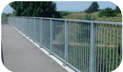
VGSP-02 A 1400mm-high steel post and vertical infill solution with posts installed at 2.0m centres.
