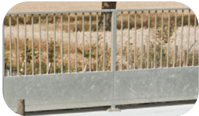
VGSP-03 A 1800mm-high steel post and vertical infill solution with posts installed at 2.0m centres. The lower 600mm is sheeted, making this ideal for bridleway and equestrian applications.
